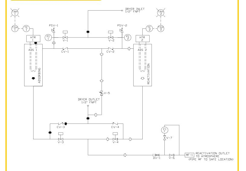
The wet gas enters the HPB Lectrodryer at the adsorption inlet. Flow is directed to the left adsorbing tower, adsorber 1, and is dried passing through the desiccant bed. The dryer gas exists through the bottom dryer outlet.
